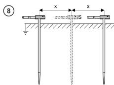
Repeat the measurements (steps 5, 6, 7) moving the voltage electrode a few meters placing it farther and closer to the measured earth electrode.
