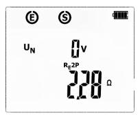
After the measurement, its result is shown: at the bottom of the screen, the main result is shown for R<sub>E</sub>2P, whereas the upper part of the screen shows the measured interference voltage U<sub>N</sub>. The result is displayed for 20 seconds. The result can be recalled by pressing ENTER button.
