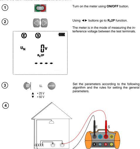
Test leads should be connected to the measurement terminals in the device, as shown above.
