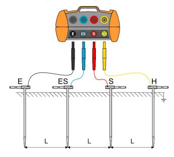
Connect the four aligned and equally spaced auxiliary electrodes, which are driven into the ground, to the meter, and do so in accordance with the diagram.
