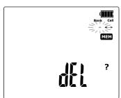
Set the bank number to • (before 0). The dtl message appears, signaling that the meter is ready to delete.
