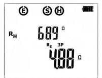
After completing the measurement, results are displayed for all the measurements carried-out: at the bottom of the screen, the main result is shown for R<sub>E</sub>, whereas the upper part of the screen shows additional results for R<sub>H</sub>. The result is displayed for 20 seconds.
