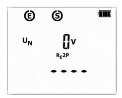
In measuring functions, before **START** button is pressed, the meter monitors the measuring voltage at the terminals (between **E** socket and **S** / **H** sockets) and the interference voltage value is displayed on the screen.
