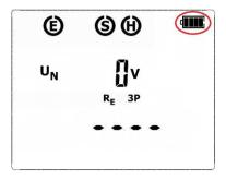
The charge level of the batteries or rechargeable batteries is indicated by the symbol in the right upper corner of the display on a current basis:
