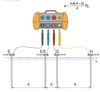
Connect the four aligned auxiliary electrodes, which are driven into the ground, to the meter, and do so in accordance with the diagram. The distance between electrodes E and ES, as well as between S and SH are equal to each other, and at the same time is greater than or equal to 3 times the distance between electrodes ES and S ( $A \ge 3 \cdot d$ ).
