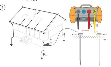
Test leads should be connected to the measurement terminals in the device, as shown above.
