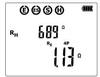
After completing the measurement, results are displayed for all the measurements carried-out: at the bottom of the screen, the main result is shown for  $R_{\text{E}}$ , whereas the upper part of the screen shows additional results for  $R_{\text{H}}$ . The result is displayed for 20 seconds. The result can be recalled by pressing ENTER button.
