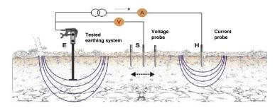
The scheme of measuring the earthing resistance with the 'technical method' is shown above. The figure shows the measurement of earthing resistance  $R_{\text{E}}$ . To perform the measurement, use two additional auxiliary electrodes:
